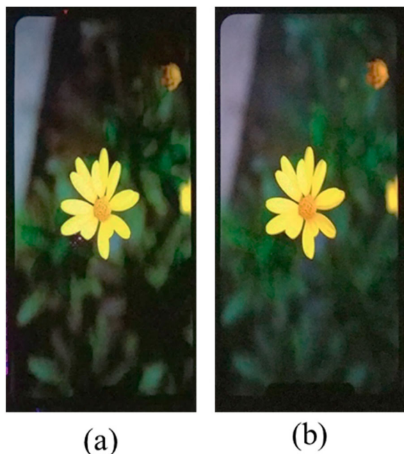
Figure 8. Improve result by minimizing of electric potential between V_{init} and V_{sat} (a) Failure image on display panel, (b) Enhancement image on 6.47" FHD+ AMOLED display panel by optimizing V_{init} .
