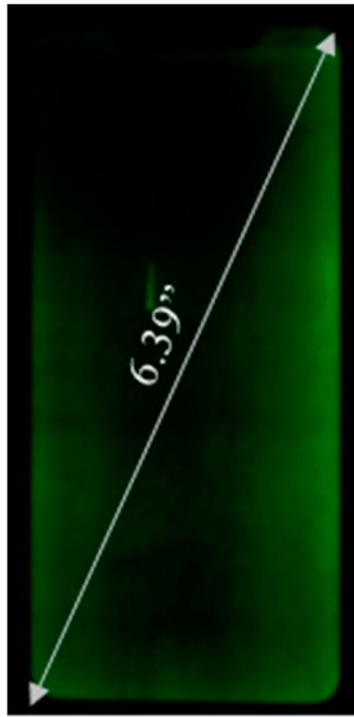
Figure 2. Example image of failure mode phenomenon on the 6.39" FHD+ AMOLED display panel at 0.02 nit (32 gray at 2 nit, 3 gray at 500nit) with the luminance difference where the panel edge areas are much brighter than the center area.
